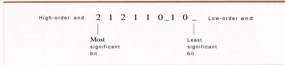
Figure 1.7 The organization of a byte-size memory cell
